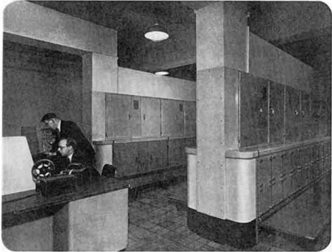
The Computer is built in two bays with a separate control desk for the operator. The machine illustrated is Model No. 1 installed at the University of Manchester.
